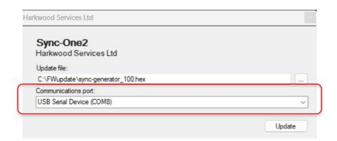
6. Press the Update button on the Firmware update tool, a progress bar will show, and Sync-Generator will flash a blue light as the firmware uploads and is verified.
